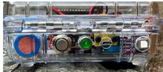
Figure 7. Power switch, reconfig switch, charging jack and CO2 sensor
