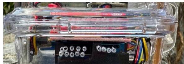
Figure 8. PM sensor outflow (left) and inlet
