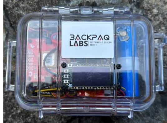
Figure 6. Display, indicator LED (upper right)
